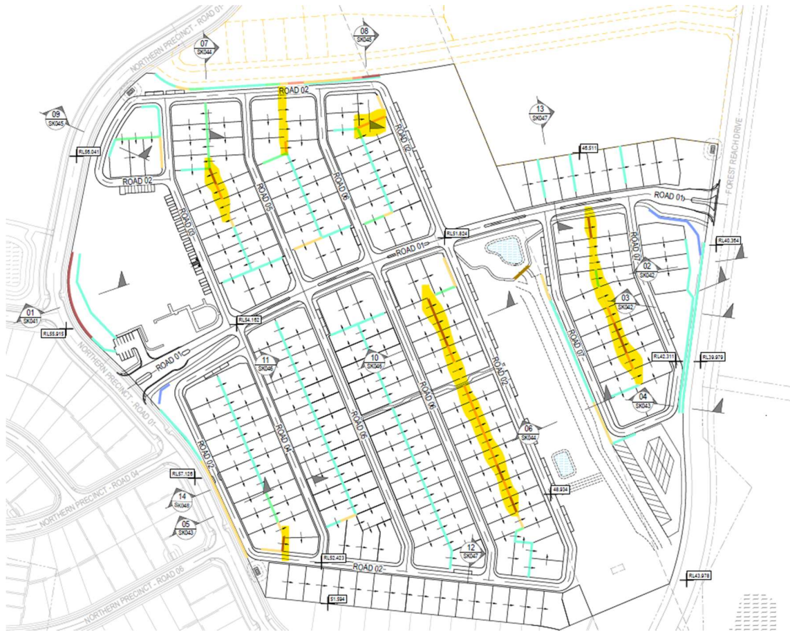
Figure 1: Highlighted retaining walls likely to result in adverse amenity impacts
